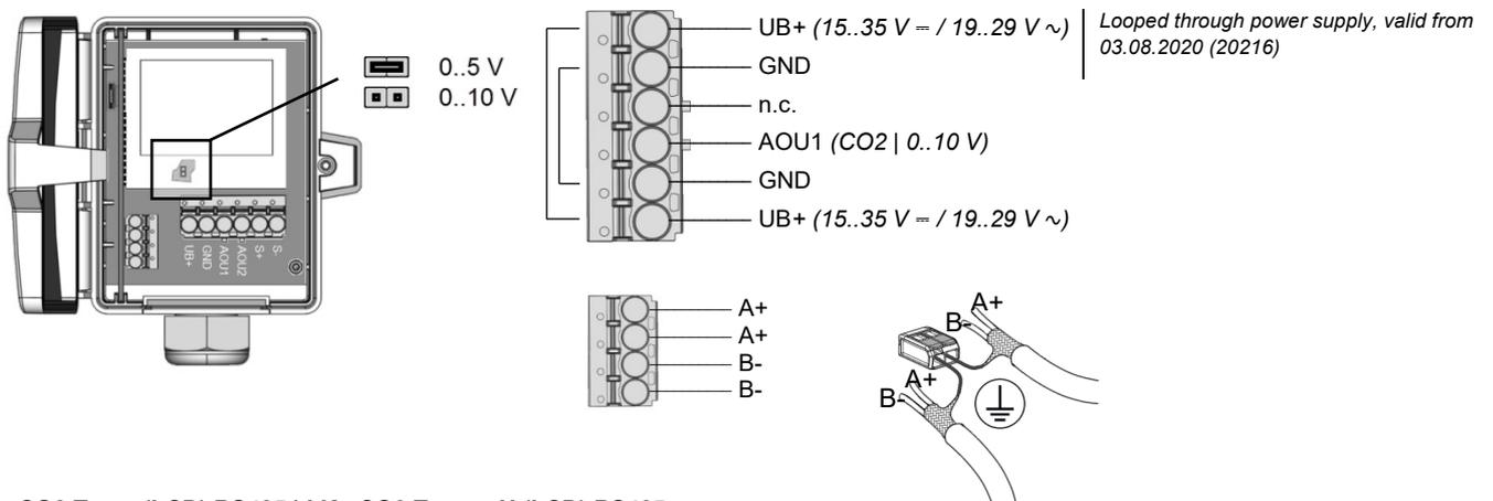
**LK+ CO2 Temp (LCD) RS485 | LK+ CO2 Temp\_rH (LCD) RS485**
