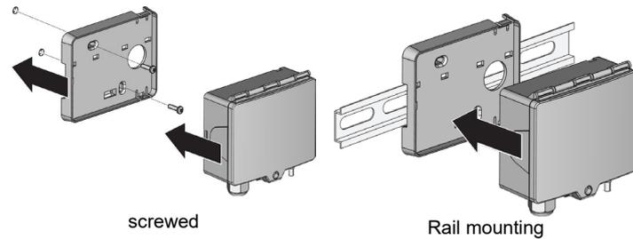
**2.** Prepare the duct for mounting and mount the duct connection piece. **Attention! Observe dimensions!**
