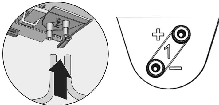
**4.** Connect pressure tubes to the duct connection pieces
