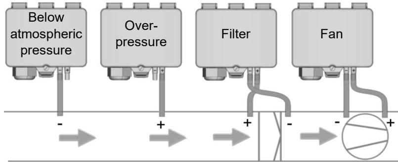
**1.** Mount the DPA+ mounting base in a suitable location and attach the DPA+. **Note alignment!**
