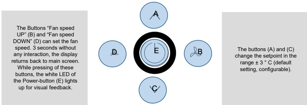
The Power button (E) can be used to switch the room thermostat to standby mode (not possible if the Keycard switch function is used!) If the key is used as a presence key at the same time, the key must be pressed for at least 3s, in all other cases a short press is sufficient. In standby mode the display and all outputs are switched off (controller deactivated). The frost and heat protection monitoring remains active. **Modbus registers can still be read (e.g. room temperature).**
