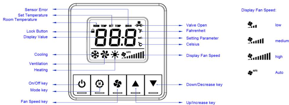
By pressing the MODE Button for more than 3 seconds, the parameter interface will appear.
