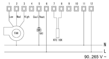
Wiring diagram for 4-pipe fan coil
