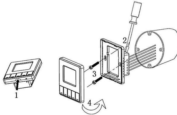
For Installing or repairing, please make sure the power is disconnected.
