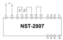
2-channel door monitoring with short circuit protection.
