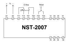
2-channel operation with external contacts, contact monitoring and short circuit protection
