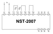
2-channel door monitoring with short circuit protection.
