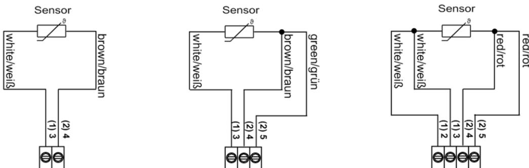
fig. (terminal assignment passive sensor)
